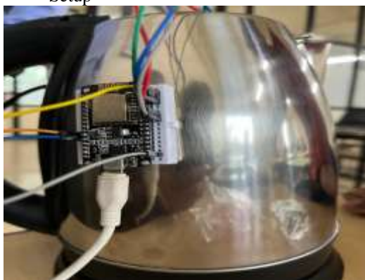
Figure 10 – Setup of the Boiling Point Monitor
